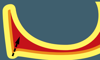
Choke: Light background extends over dark object
